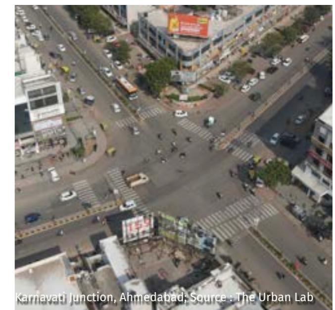
Four-leg Intersection (Crossroad) Two roads intersect at or near right angles; requires signal control and pedestrian crossings.
